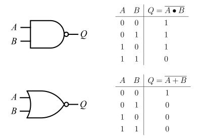
In addition to the inverter, you are also supplied with an IC containing **four** 2-input NAND gates, the MC54/74HC00A.
